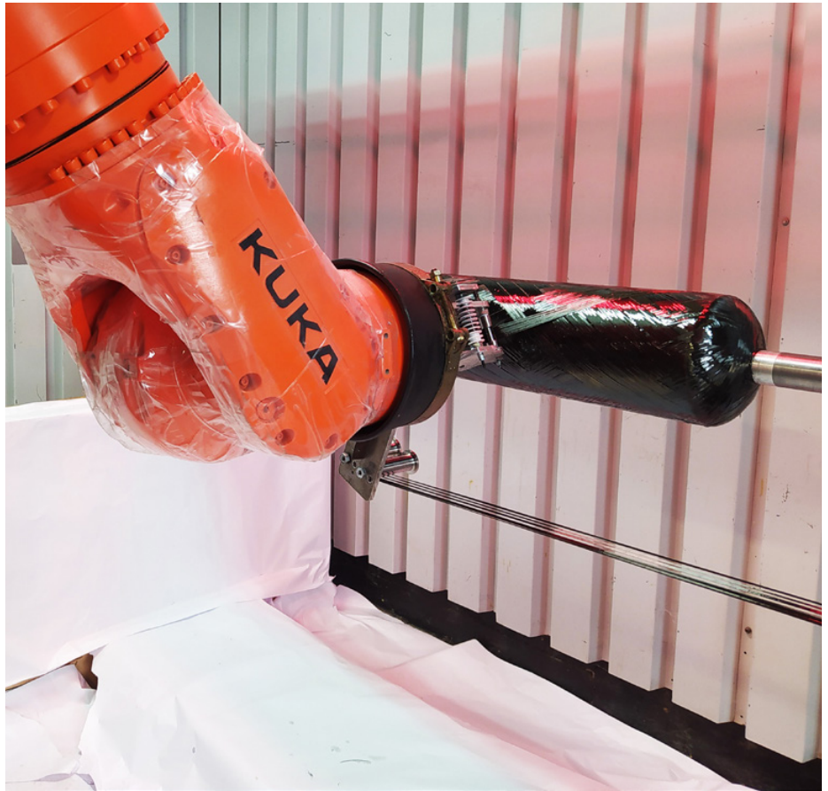
Pic. KUKA robot during tank winding.
