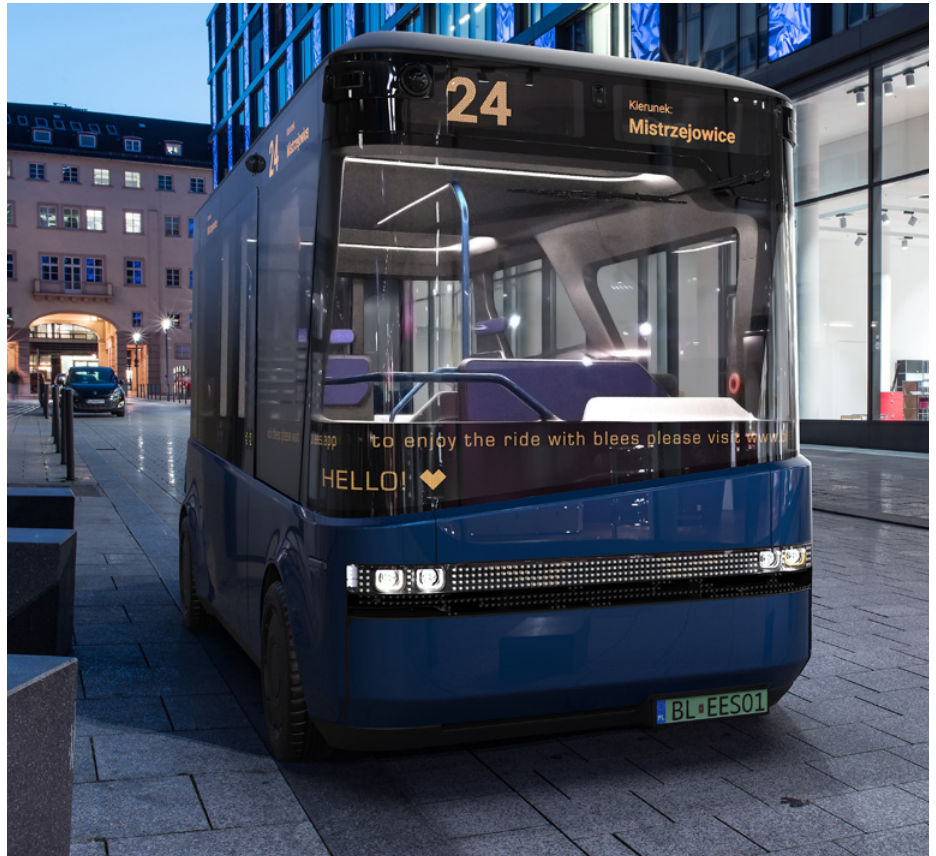
Fot. Bles – an autonomous, electric minibus
