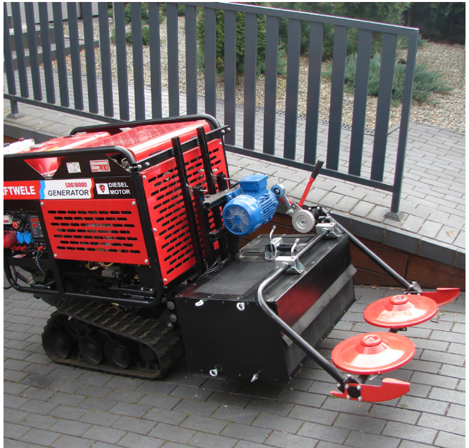
Pic. Hogweed – a device for microwave destruction of invasive plants – photo from the side
